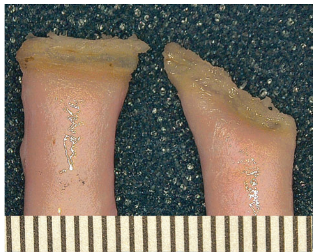
FIG. 2. Porcine carotid arteries sealed (left) perpendicularly and (right) at an angle. The scale below is 1 mm per line.
